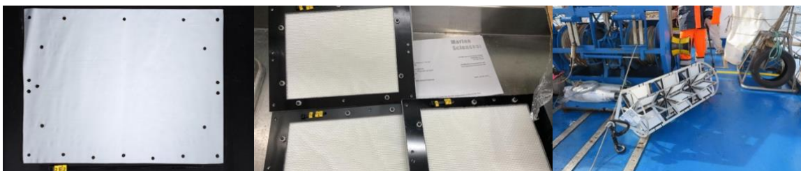
Figure 1: PHB film sample prior and post assembling in protection frames and mesh. Mounted onto steel frame ready for deployment at Sicily channel (SICO).
