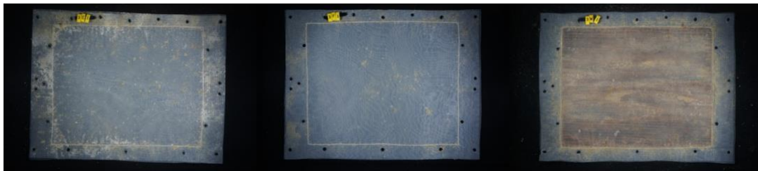
Figure 3: Documentation of samples after dismantling from protective mesh and frame. Photo documentation with the fine protective mesh: 3E1: white PHB film (100%), 3F1: white Cellulose filter paper (100%); 3W1: thin brown wood plate (0%=intact), exposed at Sicily channel (SICO).
