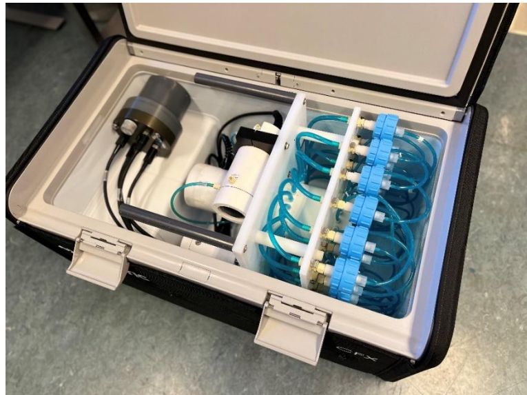
Figure 2. Modified Mclane PPS integrated in the Dometic CFX3-100 portable cooler/freezer.
