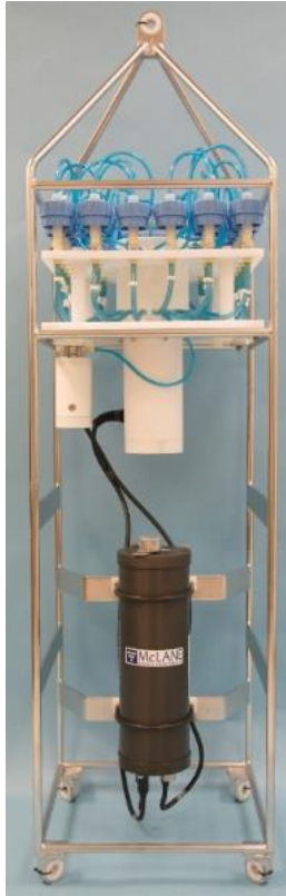
Figure 1. Mclane PPS in its original configuration (from www.https://mclanelabs.com/phytoplankton-sampler/ ).
