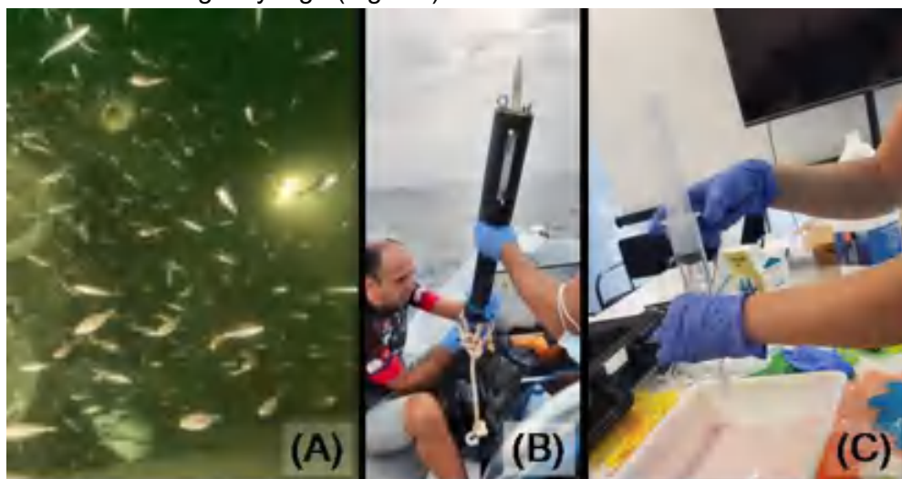
Figure 2. Image from the main camera (A), autonomous sampler (B) and syringe with sterivex filter ©
