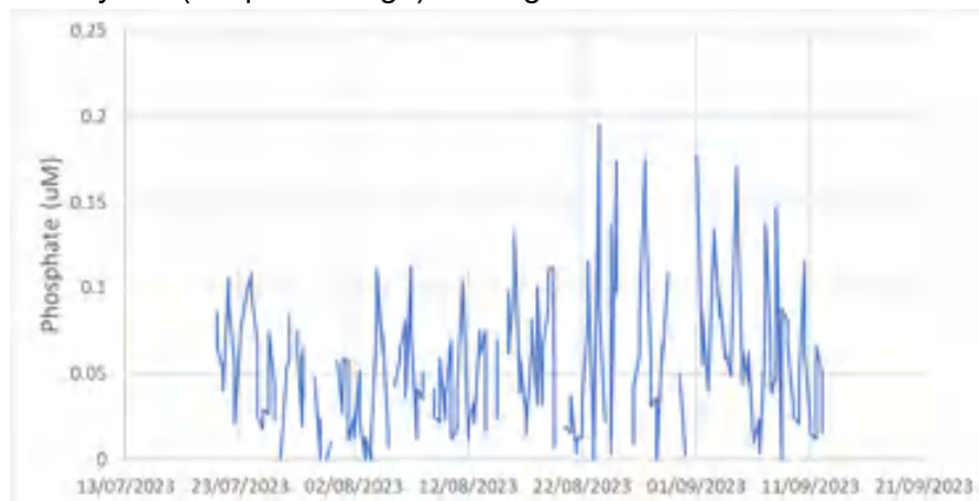
Figure 2. Concentration of dissolved phosphate in \mu\text{mol/L} , as measured by the LOC sensor at OBSEA between late July / early September 2023.
