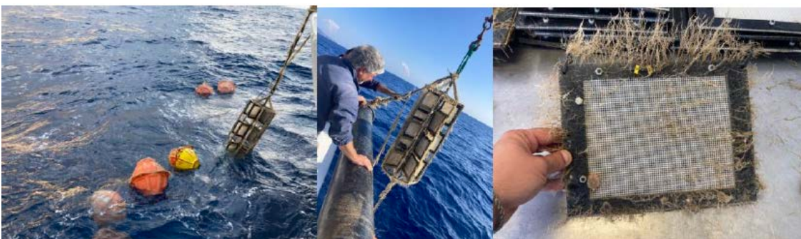
Figure 2: Retrieval of the steel frame with mounted samples at Sicily Channel (SICO) in October 2022, and documentation of fouling. All pictures are representative for the
