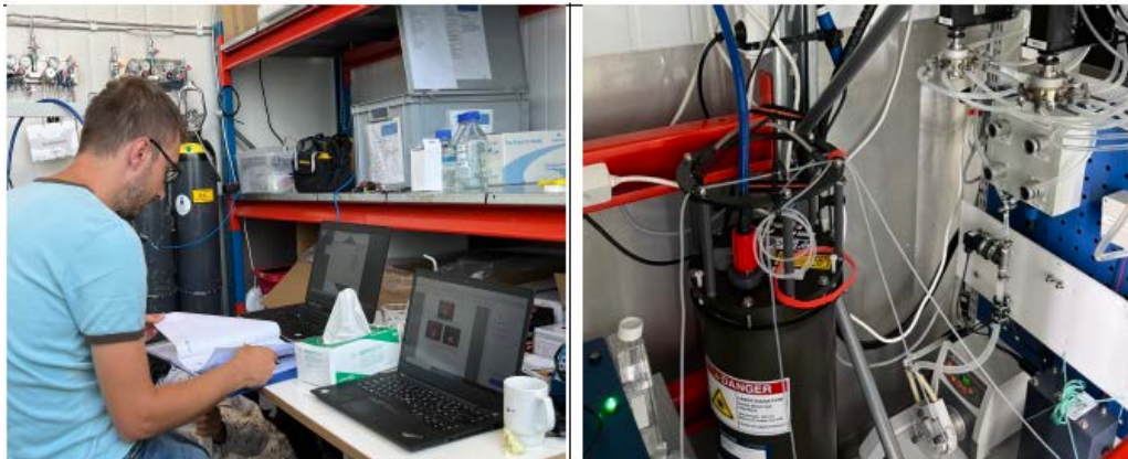
Figure 2. From left to right: Christian Dilewski trouble shooting the night measurement routine in the IFCB software; Installation of the IGB-IFCB in the AQUABOX system to run plankton samples in parallel with the SYKEIFCB (Photos: Stella A. Berger, IGB).
