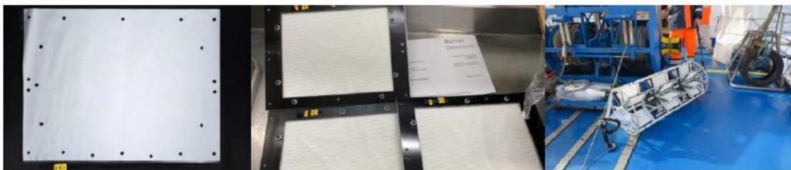
Figure 1: PHB film sample prior and post assembling in protection frames and mesh. Mounted onto steel frame ready for deployment at Sicily channel (SICO). All pictures are representative for the deployment at the Corsica Channel (CoM).
