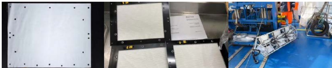
Figure 1: PHB film sample prior and post assembling in protection frames and mesh. Mounted onto steel frame ready for deployment at Sicily channel (SICO).
