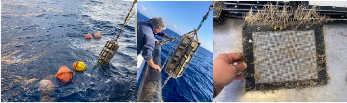
Figure 2: Retrieval of the steel frame with mounted samples at Sicily Channel (SICO) in October 2022, and documentation of fouling. All pictures are representative for the deployment at the Corsica Channel (CoM).
