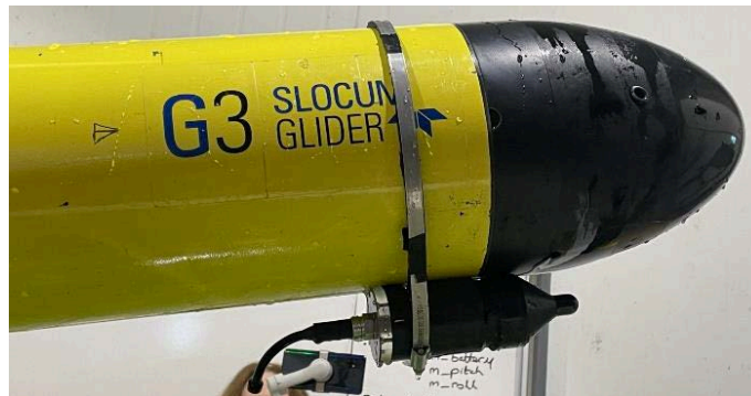
Figure 1: The soundtrap pointing forward and attached under the hull of the G3 Slocum glider.
