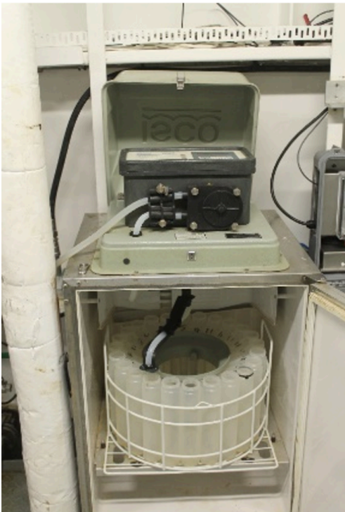
Fig. X. WASP sampling system composed of several instruments and samplers. Top: modified PPS for particulate matter sampling; Bottom left: ISCO refrigerated autosampler for water samples; Bottom right: FerryBox sensors including SeaBird SBE45 salinity-temperature and Turner Designs C3 for chlorophyll a, cDOM, and turbidity.
