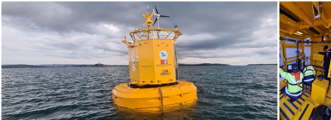
Fig. 3.1.14. Aspect of one of the oceanographic buoys in the northern Adriatic Sea (left: outside of the buoy with the city of Rovinj in the background. Right: inside of the buoy during maintenance and sensor adjustment)
