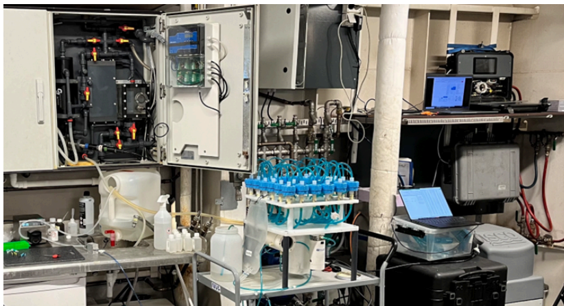
Fig. 3.1.3. The WASP sampler developed in WP7 that includes a modified Phytoplankton Particle sampler (McLane) and an refrigerated autosampler for bulk seawater connected to a FerryBox system for autonomous sampling of eDNA (photo: Anette Engesmo).
