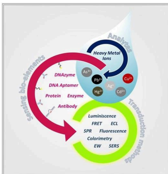
Figure 10 - Optical biosensor scheme strategies for heavy metal (HM) ion detection in water (Aloisi et al., 2019).
